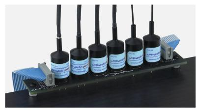
**Vertical Mounting with Standoffs:** Two stand-offs (1/4" min) are available to attach a Sensor Six-Pack to the mounting plate with screws. (Includes 2 screws and 2 standoffs) A customer supplied 4-40 screw, with a length that allows for the thickness of the mounting plate plus the available 0.156 in. of the tapped hole in the underside of the stand-off, as shown below.
