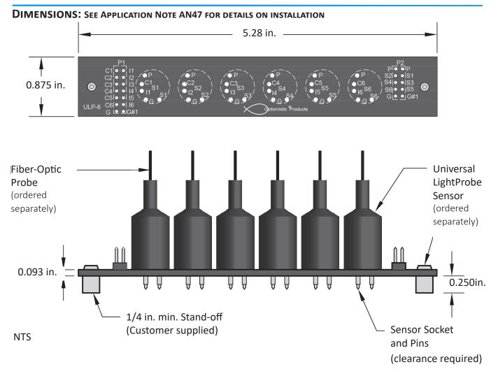
**Easy Installation**: Two tapped (4-40) mounting holes are used for installation with 1/4 in. min. stand-offs. 14-pin and 10-pin standard circuit-board header connectors accomodate analog Sensor (Penta, Spectra, Unicolor) or digital Sensor (Unicolor Digital, Blinx, UHS) outputs respectively.
