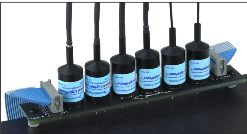
**Easy Installation:** Two tapped (4-40) mounting holes are used for installation with ¼ in./ 6.35mm stand-offs. Both 10-pin and 14-pin standard circuit-board header connectors accommodate either analog or digital Sensor outputs.
